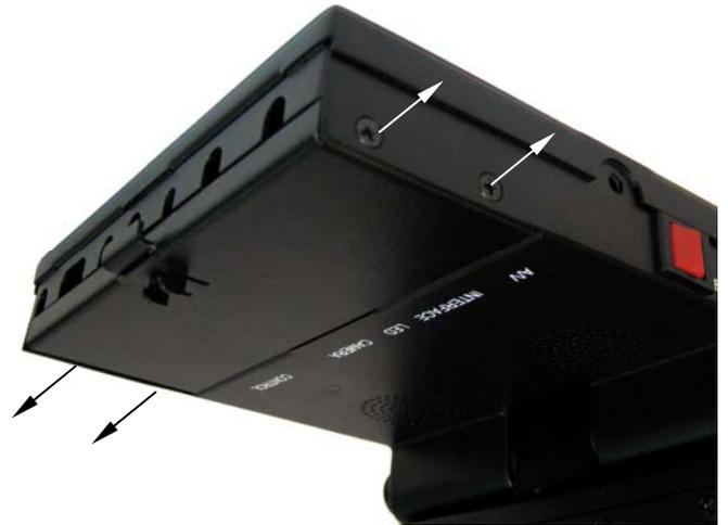
2. Remove all 4X – M3 Countersunk Phillip Head Screws using a proper screw driver.
