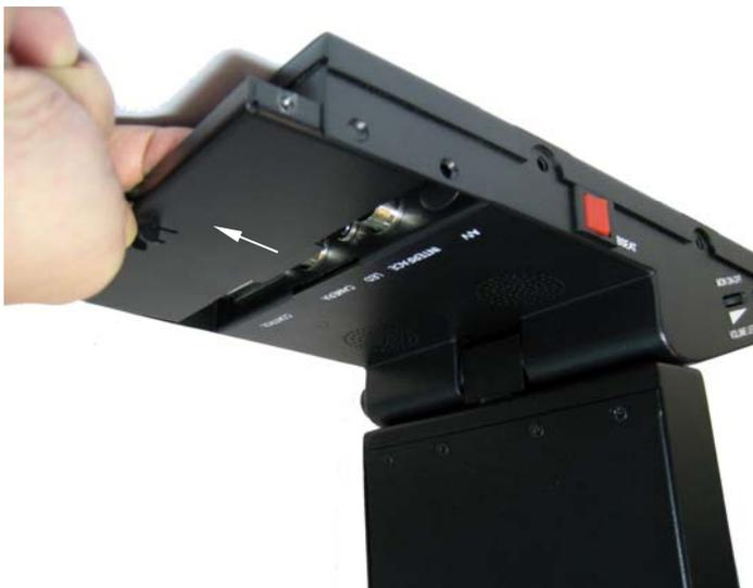
3. Slide out the wiring cover as shown above.
